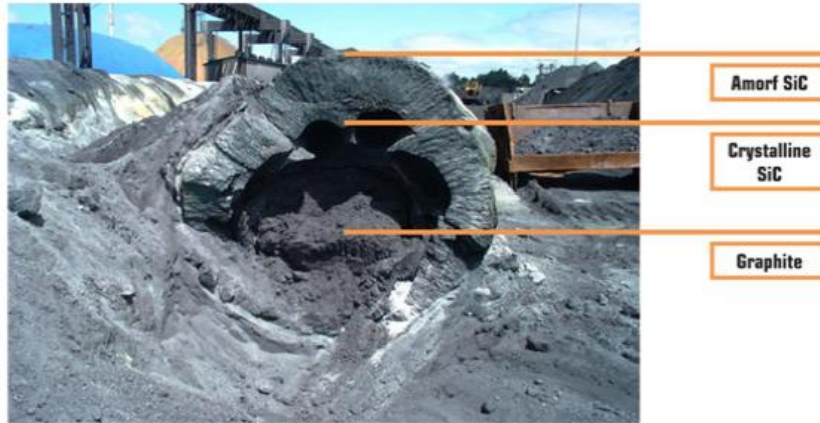
Figure 5 – Different forms of Silicon Carbide produced according to its distance to the graphite core. ESD SIC B.V., Delfzijl (ESD-SIC, 2020)
