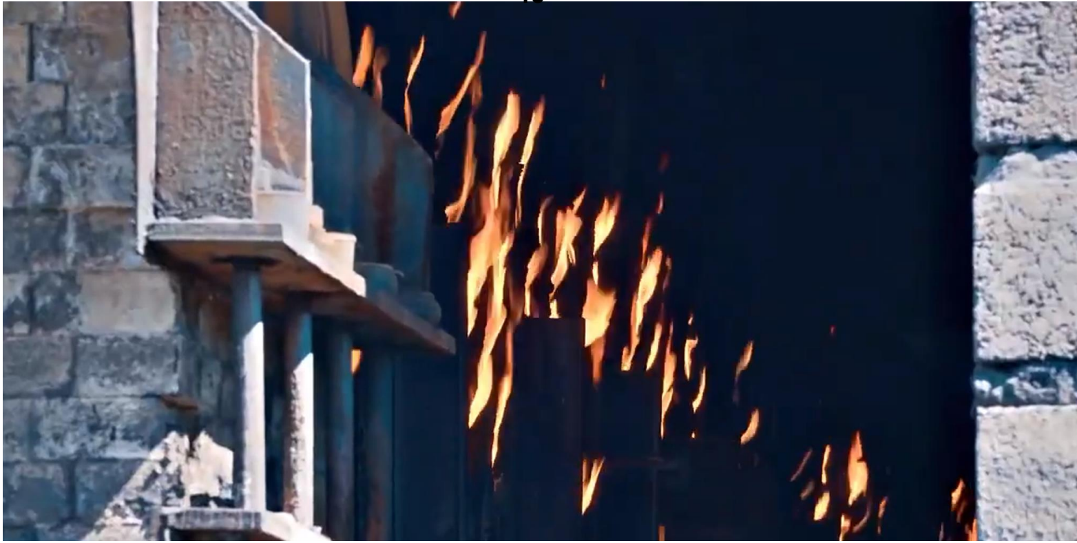
Petcoke is burning in the The Acheson furnace
